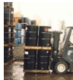
Fork lift trucks can be the source of ignition unless suitably protected.
